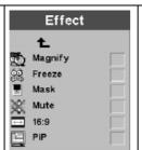
In the Effect menu, you can assign one of the displayed functions to the "Effect" button on the remote control. You can select only one of these functions at a time.
